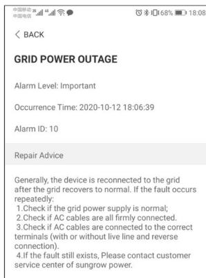
figure 7-9 Detailed Fault Alarm Information
