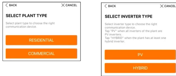
figure 6-3 Selecting Plant/Inverter Type
